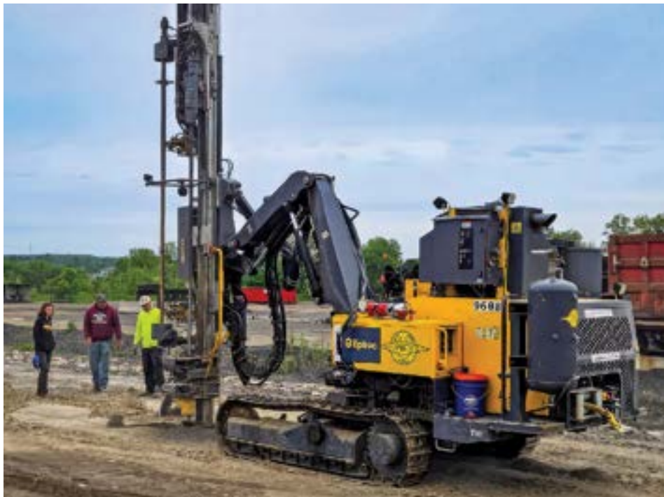
This spring, the Epiroc Drill Rig was stationed at the New York Training Center, where Instructors Terrence O'Brien Jr. and Bucky Rocco led hands-on training sessions. The drill is used to bore holes for solar array foundations. Members trained on the rig are gaining the skills and certifications needed to operate it safely and effectively in the field.
