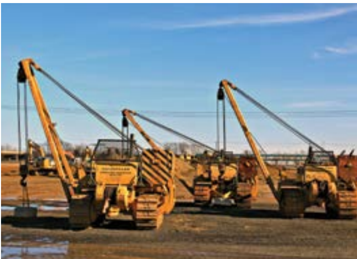
Side Boom Pipeline Class participants familiarize themselves with the boom controls and the brakes.
