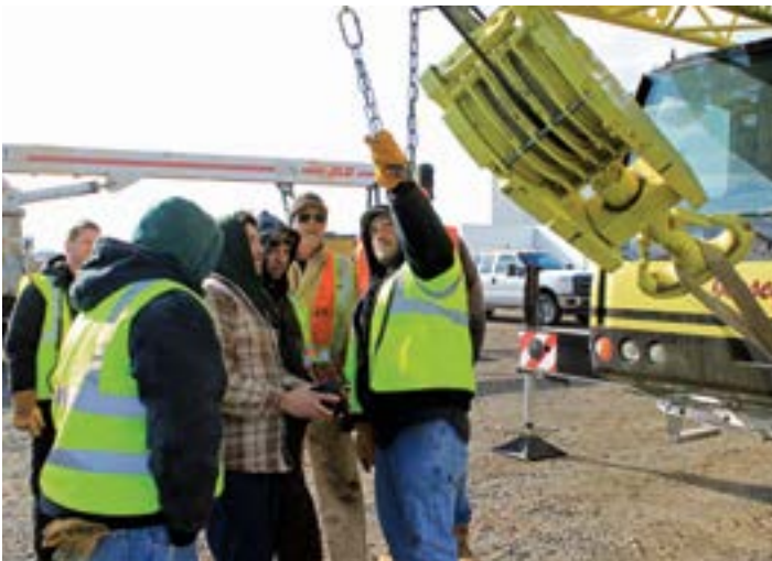
Chris Moglia demonstrates to the Basic Crane class members how to test the tube lock.
